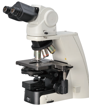
Ci-L configured with phase contrast accessories
