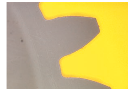
Plastic Gear Teeth with Smaller Module
